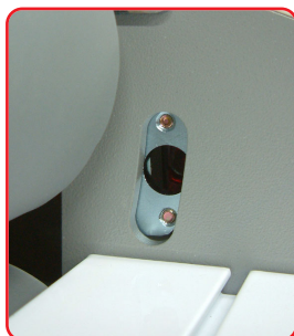
③ Safety Sensor Positioned right and left side between front table and upper roller. Equipped for user's safety and prevention of trouble when alien substances, part of user's body or necktie will be rolled into roller during operation.
