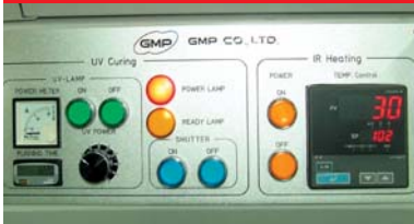
UV Control Panel
